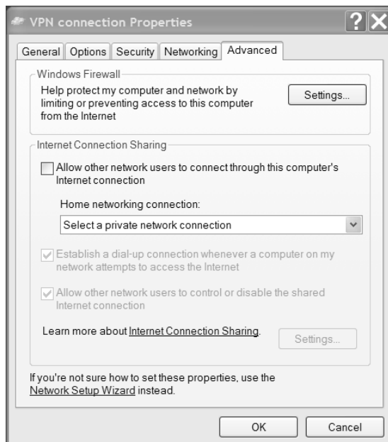
FIGURE 6.22 The Advanced tab of the VPN Connection Properties dialog box
