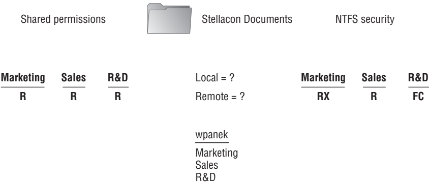
FIGURE 8.7 NTFS security and shared permissions example
