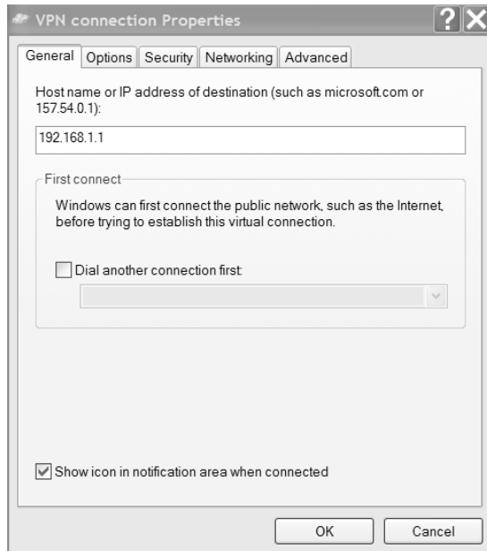
FIGURE 6.18 General tab of the VPN Connection Properties dialog box
