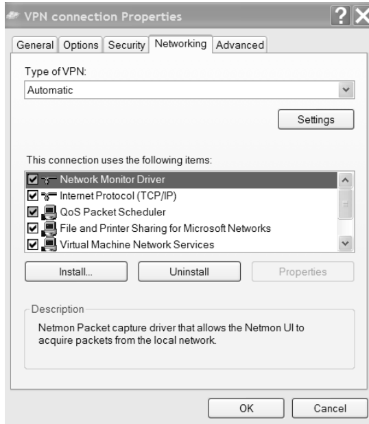
FIGURE 6.21 Networking tab of the VPN Connection Properties dialog box
